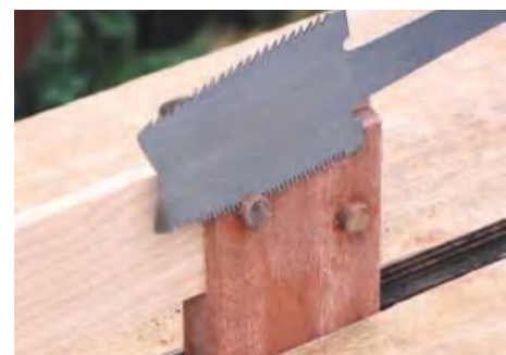
▲ The finer teeth are also ideal for sawing dowels flush or cutting smaller dimension timber
